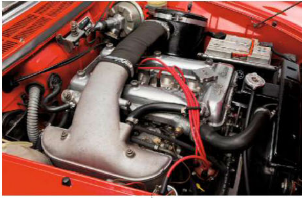
Engines range from 1.3 to 2.0 litres – all are straight-fours with a crossflow twin-cam cylinder head and are reliable and fizzy performers if well maintained
